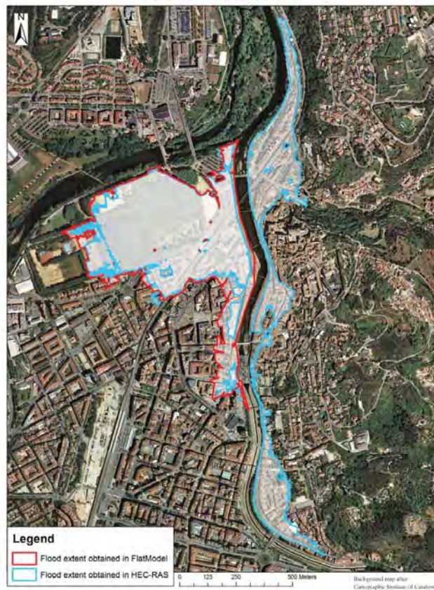
Figure A.51. Comparison of the flood extent obtained in HEC-RAS 1D/2D modelling and in 2D FLATModel for 100 years flood return period
